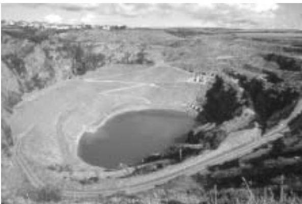
Figure 5 Delabole slate quarry in 1993, which has been worked continuously since at least the 16th century. The lower part of the quarry has been allowed to flood and working is now concentrated on the right hand side. (c. Colin Bristow)
