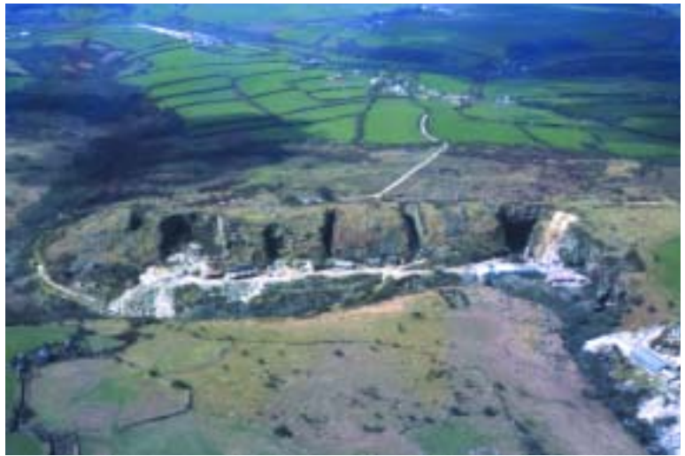
11. De Lank Granite Quarry, St Breward. A dimension stone and aggregates quarry that has eaten into a low ridge. On the left is Eddystone Quarry which provided the stone for the lighthouse. A railway incline took stone down to the Bodmin and Wadebridge Railway terminus at Wenford (in the valley at the top of the photo). Site survey: Cornwall Archaeological Unit 1993 published in Herring et al. (forthcoming). (c. Historic Environment Service, Cornwall County Council)
