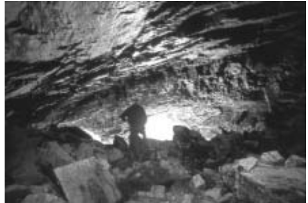
Figure 6 Underground working for limestone at Trenault, near Launceston. The limestone is a condensed sequence ranging from the uppermost Devonian into the lowermost Carboniferous. Conodont microfossils enable this limestone to be correlated with other limestones of this age in SW England and on the Continent. Most of the limestone from this mine was used for lime burning. (c. Colin Bristow)
